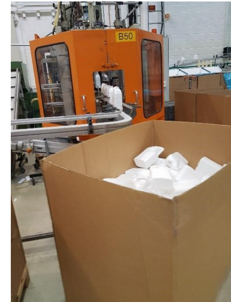
Heat-Extrusion-Moulding machine for white bottles
